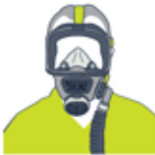
Figure 4: PPE; full-face powered respirator (for high dust levels or people with facial hair)
